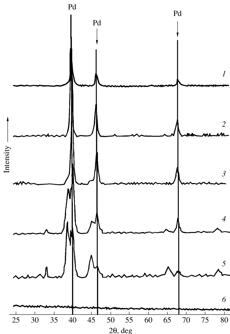
Fig. 3. Diffractograms of the catalysts 5%Pd/SiO 2 , 5%Pd1%Tl/SiO 2 , 5%Pd3%Tl/SiO 2 , 5%Pd5%Tl/SiO 2 , 5%Pd8%Tl/SiO 2 , and 5%Tl/SiO 2 . Crystalline phases were identified by references to the ASTM data files.
